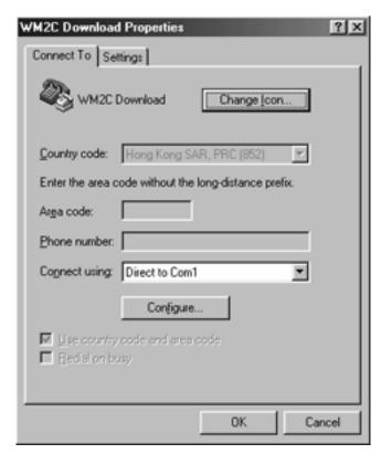
Press the "Configure" button (just under the communication port). The "COM1 Properties" dialog box appears.
