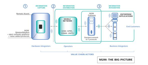
The Wavecom approach is designed to enable customers to make their business processes more efficient by using wireless technology to integrate M2M applications into end-to-end enterprise IT systems. This happens in three phases:
