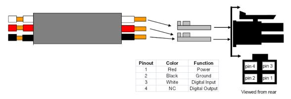
Figure 5-4: Power Connector Diagram
