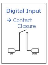
Figure 5-2: Digital Input Contact Closure
