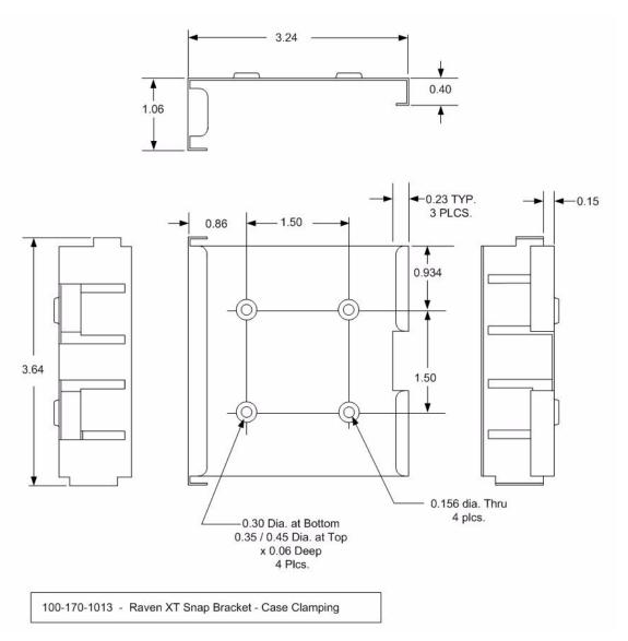
Figure 4-7: 100-170-1013: Mounting Bracket for Raven XT
