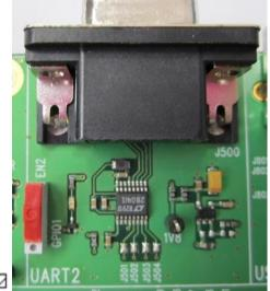
Figure 15. Enable UART2 Configuration
