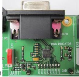
Figure 13. Enable UART1 Connector
