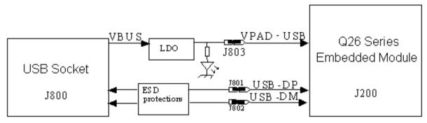
Figure 20. USB Electrical Diagram
