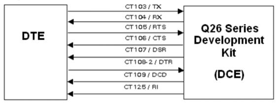
Figure 14. RS232 Main Serial Link
