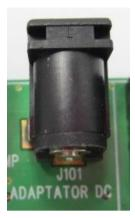
Figure 6. Main Supply Adapter
