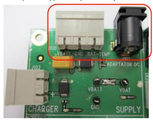
Figure 3. Power Supply Voltage (J101 and J102)
