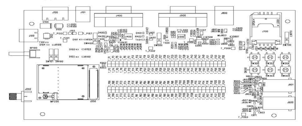
NOTE: The SMA connector (J202) and the IMP connector are not mounted.
