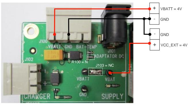
Figure 26. Configuration for the Current Measurement
