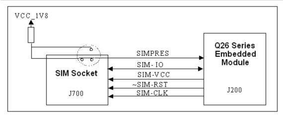
Figure 18. Schematic Diagram of the Switch "SIMPRES"
