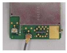
Figure 25. UFL Connector for use with a GPS Antenna
