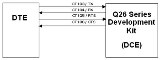
Figure 16. RS232 Auxiliary Serial Link
