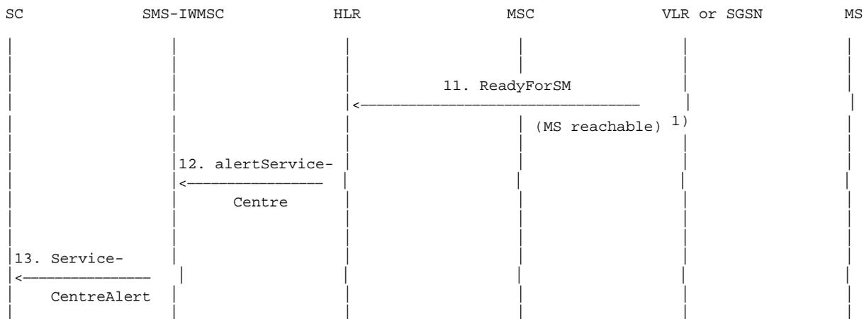
**Figure 03.40/20a: The alert procedure when the MS becomes reachable, MNRF, MNRG or both are set and MCEF is not set**
