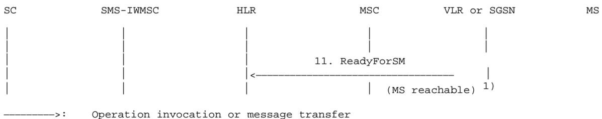
**Figure 03.40/20b: The alert procedure when the MS becomes reachable, MNRF, MNRG or both are set and MCEF is set**
