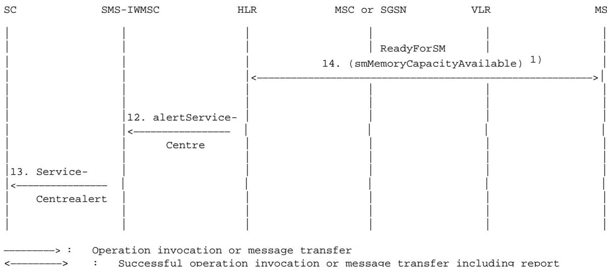
**Figure 03.40/20c: The alert procedure when the MS notifies the network that it has memory available to receive one or more short messages and MCEF is set**
