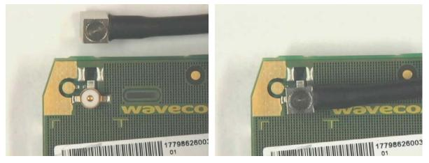
Figure 6: Assembly process - MMS connector
