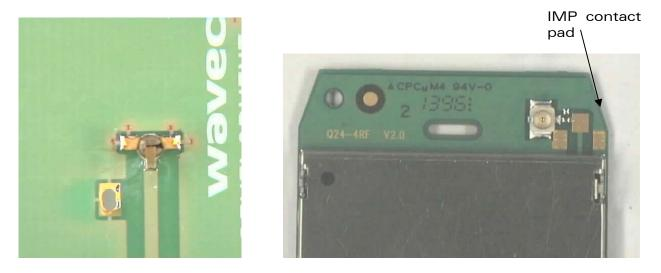
Figure 13: Assembly process - IMP connector
