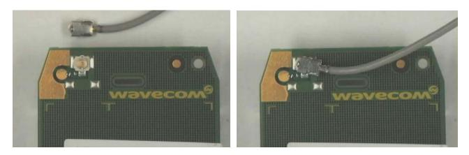
Figure 10: Assembly process - UFL/SMA connector
