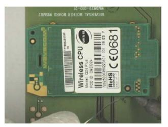
Turn the application board and solder the 4 legs on this side.
