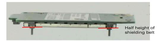
Figure 18: Assembly process - Half height of shielding belt
