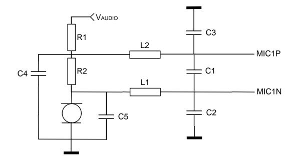
Note : VAUDIO must be very "clean" in single-ended connection (for example, VCC plus filter cell like RC or LC).
