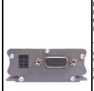
Fargo Maestro 100 and Fargo Maestro 100Lite (GPRS Class 10) are external Industrial dual band GSM modems in 900/1800 MHz. Powered by the FRENCH TECHNOLOGY from WAVECOM. They can be quickly connected to the serial port of a desktop or notebook computer through their RS 232 interfaces for remote connections.
