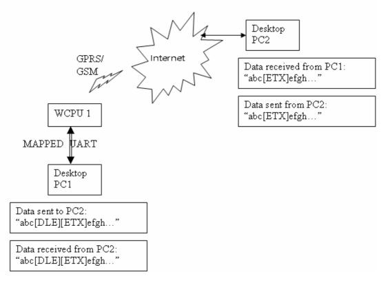
The above schematic explains how [ETX] characters - which have a special meaning in WIP soft - are handled on Wavecom Wireless CPU<sup>®</sup>. On transmitting side, when [ETX] are not escaped (use case: Desktop PC1 sends data towards Wireless CPU<sup>®</sup>. Data contain a non escaped [ETX] (⇔ no [DLE][ETX] sequence), then [ETX] is not transmitted but an action is done on Wireless CPU<sup>®</sup> regarding the concerned socket:
