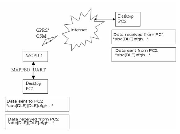
The above schematic explains how [DLE] characters - which have a special meaning in WIPSoft - are handled on Wavecom Wireless CPU<sup>®</sup>.
