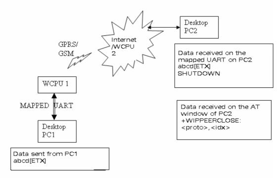
In the above schematic, a TCP socket is connected. On the transmitting side, data and [ETX] is sent (use case: Desktop PC1 is a Wireless CPU® which sends data to PC2 which is either a PC or a Wireless CPU<sup>®</sup>), the data is received on PC2 and [ETX] character shutdowns the socket on the transmitting side and displays a message "[CR][LF]SHUTDOWN[CR][LF]" on the mapped UART of PC2.
