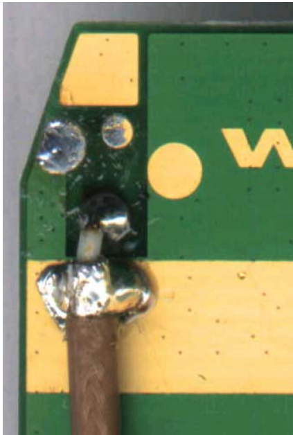
Figure 9a: Coaxial cable soldered on the top of the 2D module
